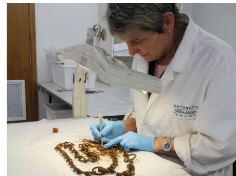
Conservator Sue Bassett removes corrosion from iron dog chains.
