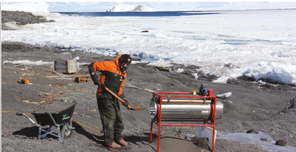
Dusty scoria from the stables at Cape Evans being fed into the trommel. © AHT/AI Fastier
