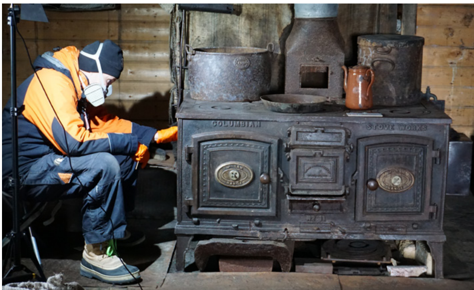
Megan Absolon undertakes solubility tests on the stove in Shackleton's 'Nimrod' hut for the purpose of informing future treatment options. © AHT/Jane Hamill
