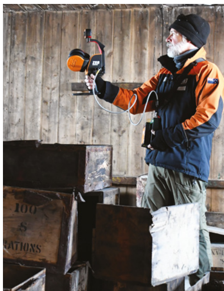
Gord Macdonald using a portable laser scanner to scan the interior of Scott’s Discovery hut. ©AHT/Zack Bennett
