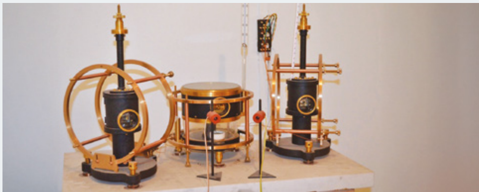
La Cour magnetograph sensors donated to the Trust by GNS Science. © GNS Science
